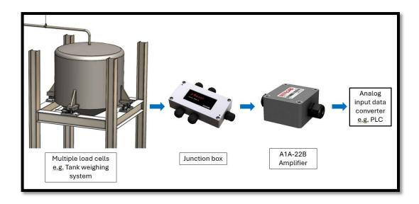
Connect the load cell/junction box, power supply and the analogue data input devices to the amplifier board as per below schematic diagram.
